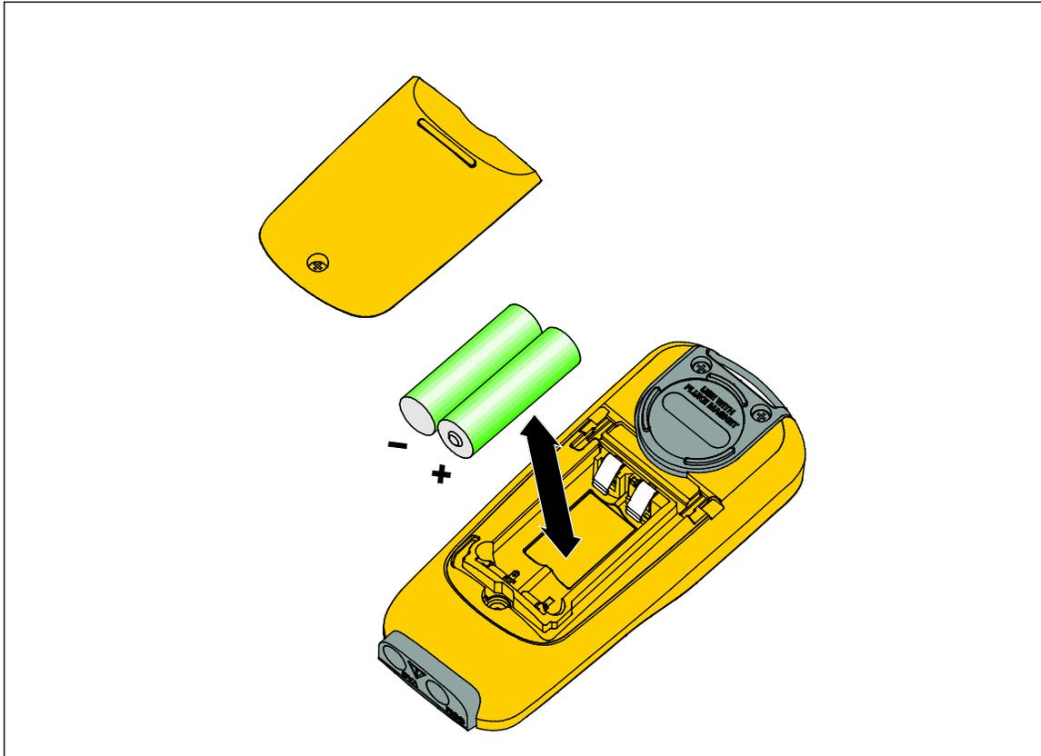
Figure 4. Battery Replacement
