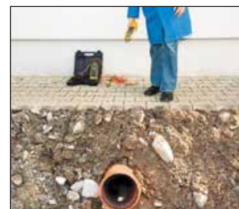
Tracing of underground cables (max. depth 2.5 m)
