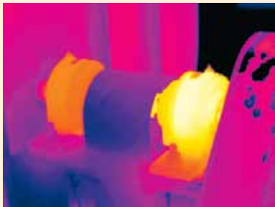
Overheating bearing cap
