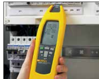
Location of fuses/breakers and assignment to circuits
