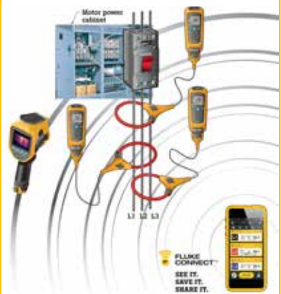
Three-phase unbalance testing with Fluke Connect Wireless Tools
