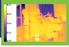
This nitrogen pump had a persistently leaky seal and had to be changed out regularly. Thermal imaging revealed a restriction preventing the seal from receiving enough cool airflow. As a result, the seal was overheating and melting.
