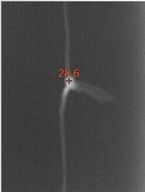
The temperature quickly went from 23.3 °C to 28.6 °C when the knot was subjected to the maximum tractive force.
