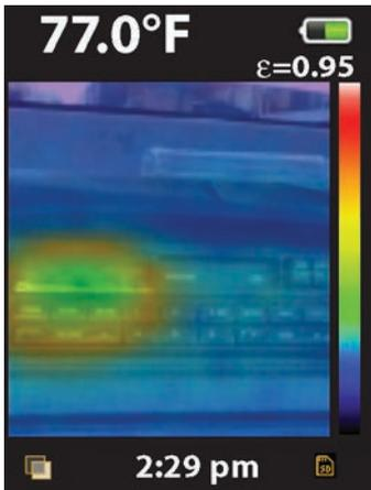
This radio was diagnosed without pulling it out of the dash. With the key turned-off, the left side indicated current draw draining the battery, warranting further investigation with a current clamp. The diagnosis proved to be a defective radio.
