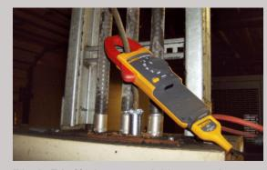
Using the Fluke 381 clamp meter, technicians measured a significant amount of ground current flowing from each air compressor. Photo courtesy of Linamar Corporation
