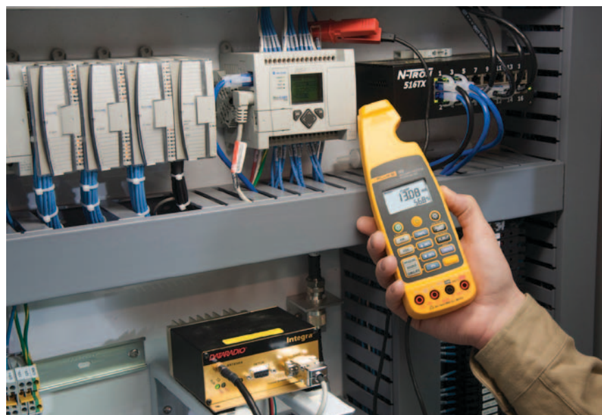
Figure 4. Measuring current on a 4–20 milliamp process control loop.
