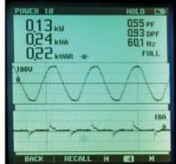
**CFL voltage and current.** While the voltage is a sine wave, the current is used in narrow pulses. As a result the crest factor (CF) reading for the current is 4.0, meaning the peak current is 4 times the rms value rather than the desired 1.4 of an undistorted sine wave, as appears in the voltage above.
