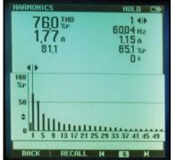
**CFL power statistics.** The kW reading is much lower than the kVA reading because current harmonics cause the total power factor (PF) to be much lower than the displacement power factor (DPF). DPF indicates the slight lag of fundamental current from the voltage.
