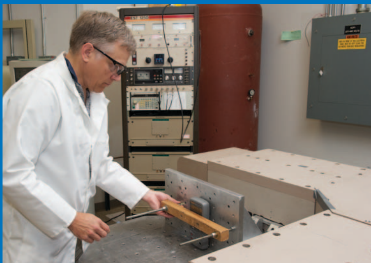
A meter is strapped in place for vibration testing.
