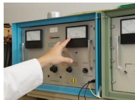
The dielectric test verifies that current can't escape the meter's shell.
