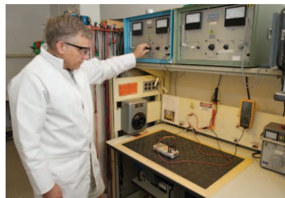
The dielectric test verifies that current can't escape the meter's shell.
