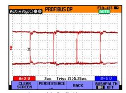
Figure 2. After making corrections to the Profibus network, new screen images of the Bus Health parameter screen (left) and the eye-pattern screen (right) were recorded. These clearly show improved network performance, with all parameters meeting requirements and well formed square wave pulses.
