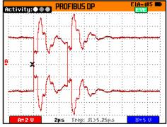
Figure 1. Left: The overshoot reading at this station is so high that an error in the network is likely and calls for further investigation. Right: The alternative way of looking at the bus signals using the eye-pattern mode shows that pulses are largely distorted, making it clear that there is an aberration on the signal at this location.
