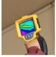
Thermal Imagers are becoming indispensible for identifying airflow and moisture problems and air leaks by their tell-tale changes in temperature. By using a thermal imager to scan a building, techs can quickly zero in on problem areas and then investigate further with other tools.
