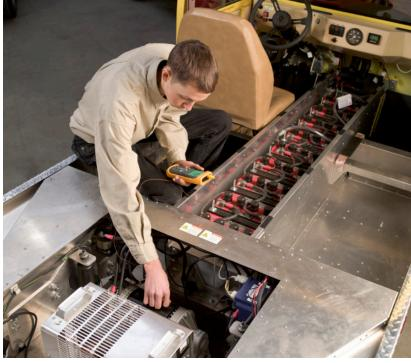
Monitoring motor temperature on an e-ride EXV-4.
