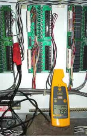
**Figure 2:** In specific applications, percentage readings on the Fluke 771 may be more useful than the underlying current readings – for example, when a control output must be maintained within a range of 25-30 % of the maximum level. Here, the Fluke 771 is connected to the emission control loop.
