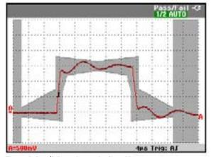
Figure 4. Pass/fail template at the ScopeMeter.
