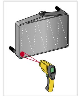
**Fig. 5** Scan along target to locate higher temperature areas.
