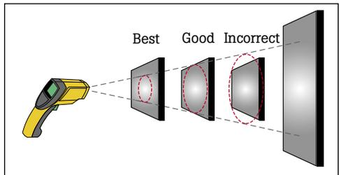
**Fig. 4** The target should be larger than the spot size the unit is measuring.
