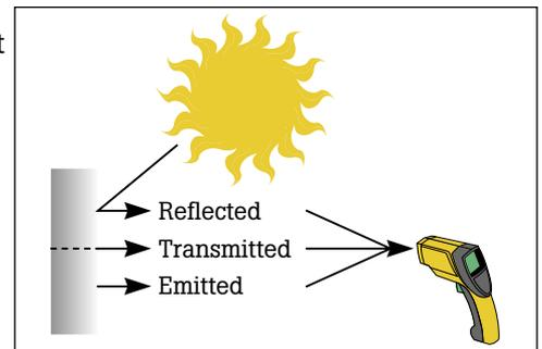
**Fig. 2** Only the emitted energy indicates the temperature of the object.
