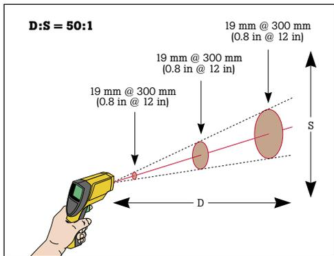
**Fig. 3** Optical resolution is the ratio of the distance from instrument to the object compared to the size of the spot.
