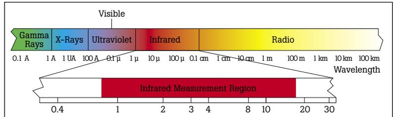
**Fig. 1** IR thermometers capture the invisible infrared energy.
