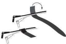
2. Loop (wrap) the strap around the rolled up leads to secure the bundle.
