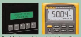
Figure 4. Output frequency (motor speed) using the low pass filter.
