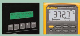
Figure 2. Output voltage reading with low pass filter enabled.
