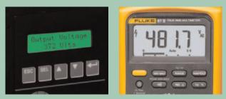
Figure 1. Output voltage reading without using the low pass filter.
