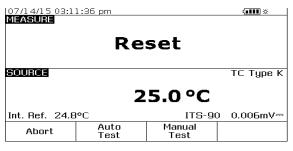
Figure 5. MEASURE/SOURCE split screen, contacts reset.
