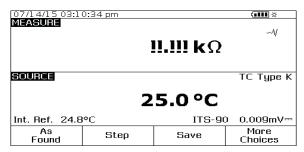
Figure 2. MEASURE/SOURCE split screen, contacts open.
